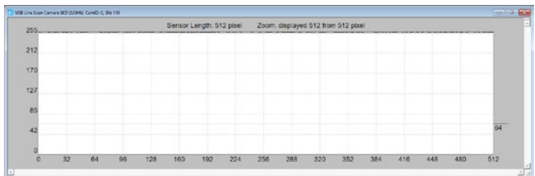
Fig. 4 Line scan signal with a homogeneous intensity at 255 (8 bit, Maximum 100%) after shading correction
