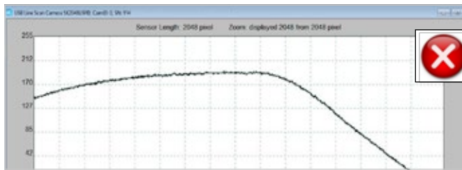
Sensor and line lighting slightly twisted in relation to each other, asymmetric vignetting
