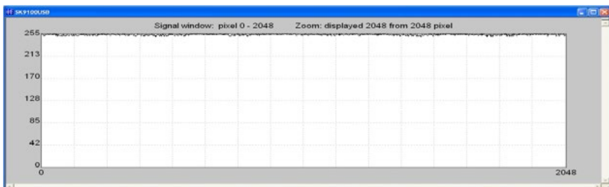
After shading correction, the line scan signal has a homogeneous intensity at 255 (8 bit, Maximum 100%)
