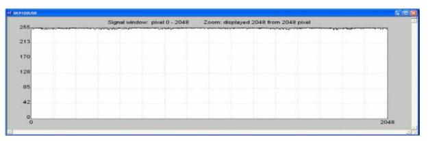
After shading correction, the line scan signal has a homogeneous intensity at 255 (8 bit, Maximum 100%)
