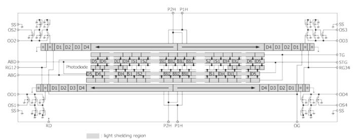
Schematic of CCD chip
