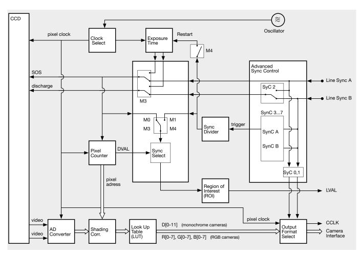
Functional diagram of the Camera Control System
