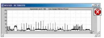
A camera signal with insufficient level: The integration time is too short, since only about 50% of the gray levels are used.
