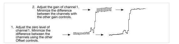
Offset and gain adjustment for more than one gain/ offset channel
