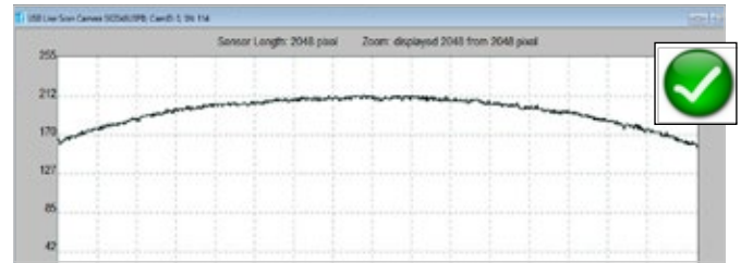
Sensor and line lighting aligned in parallel, symmetric vignetting
