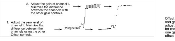
Offset and gain adjustment for more than one gain/ offset channel
