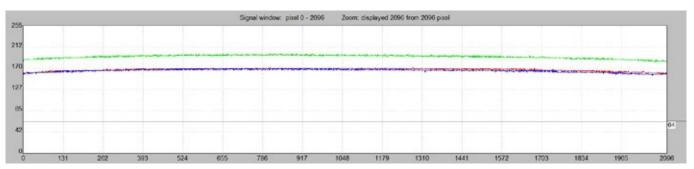
Color line signal with the Red signal adjusted to that of the Blue channel; the Green channel is still separate
