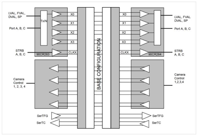
Block Diagram of Camera Link Base Configuration
