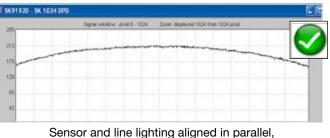
nsor and line lighting aligned in paralle symmetric vignetting
