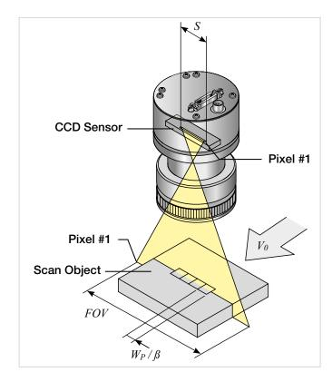
The optimal scan speed for a given line frequency is calculated as follows:
