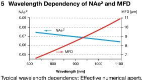
Typical wavelength dependency: Effective numerical aperture  $NAe^2$  (left scale) and mode field diameter *MFD* (right scale) as a function of the wavelength for a PMC-780 fiber.
