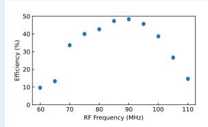
Tunability measurement for a prototype at 561 nm and a center radio-frequency of 80 MHz (MT-80-B30A1-VIS, AA Optoelectronics). Double-pass AOM efficiency  $P_{out}/P_{in}$  for different RF frequencies measured behind the output fiber (all values and data are preliminary).
