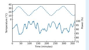
The ambient temperature is varied between 10 °C and 35 °C in a climate chamber with a cycle time of roughly 130 minutes (dashed line).
