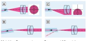
Matching ComponentsComponent MismatchCollimation A and fiber-coupling using couplers with<br/>inclined coupling axis. Mismatching collimator C and<br/>coupler D.
