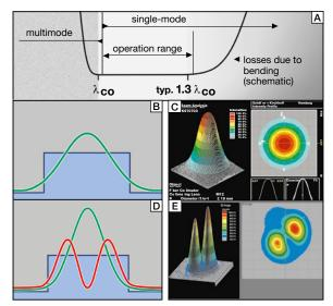
Operating range of a single-mode fiber  $\boxed{A}$ Gaussian Mode field of a single-mode fiber  $\boxed{B}$  and resulting Gaussian intensity distribution  $\boxed{C}$  at the fiber exit. Fiber used below the cut-off wavelength (here 780 nm): At 633 nm the mode field shows multiple modes (butterfly effect)  $\boxed{D}$ , which results in a non-Gaussian intensity distribution  $\boxed{E}$ .
