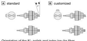
Orientation of the 8°- polish and index key for fiber connectors of type FC-APC: A standard, B optional customized orientation (FCP8).
