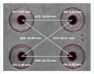
Using the linear scanner system from Schäfter+Kirchhoff, the measurement of distances, dimensions and positions of objects is possible.
