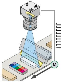
The production of a 2D image requires precise synchronization of the line camera sensor and the speed of transport of the object.
