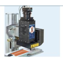
Measurement and evaluation of corrosion phenomena on coated test panels
