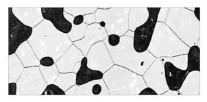
Scan of an ice core from a depth of 60 m under Antarctica. The light granular structure and dark gas bubbles are clearly discernable.
