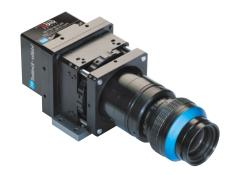
Line scan cameras are semiconductor cameras used in many industrial environments. The single photosensitive line sensor contains – depending on type – up to 22800 picture elements (pixels). Light energy incident on the sensor is transformed into an electric signal for digitization within the camera.
